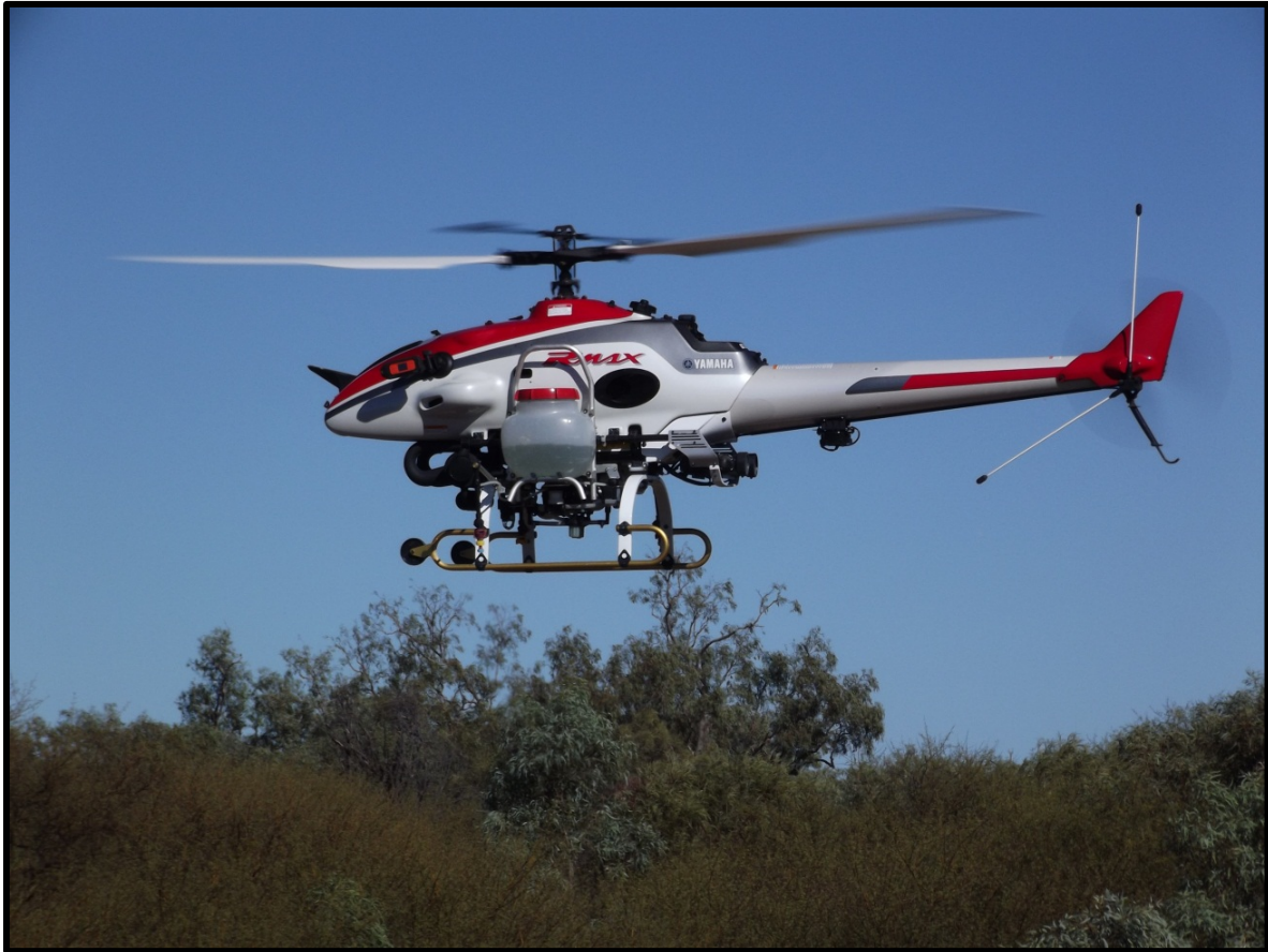
Figure 3 – UAV Operated by PBE Pty Ltd configured for foliar spraying.
