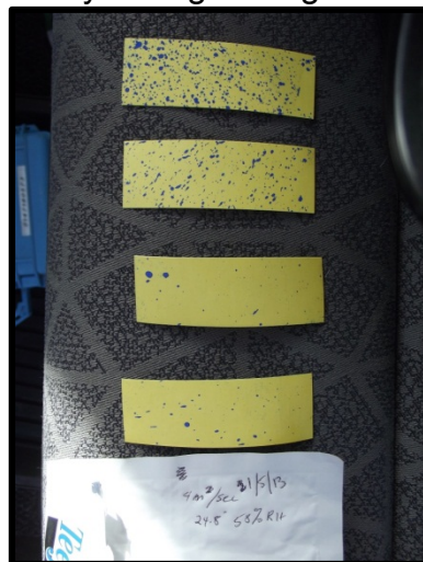
Figure 2 – Water sensitive paper used to test different application speeds and heights.
